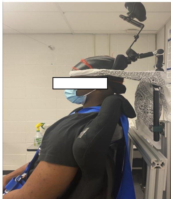
Figure 4.1. Participants head secured into the head rest utilizing bandannas
