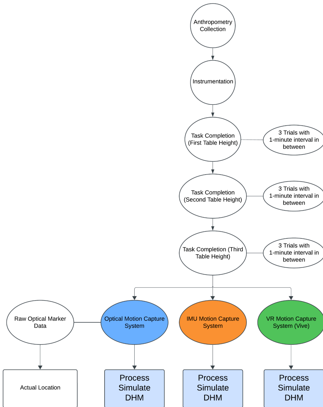
Figure 3.3. Experimental Protocol in chronological order, including the flow of data into the DHM.
