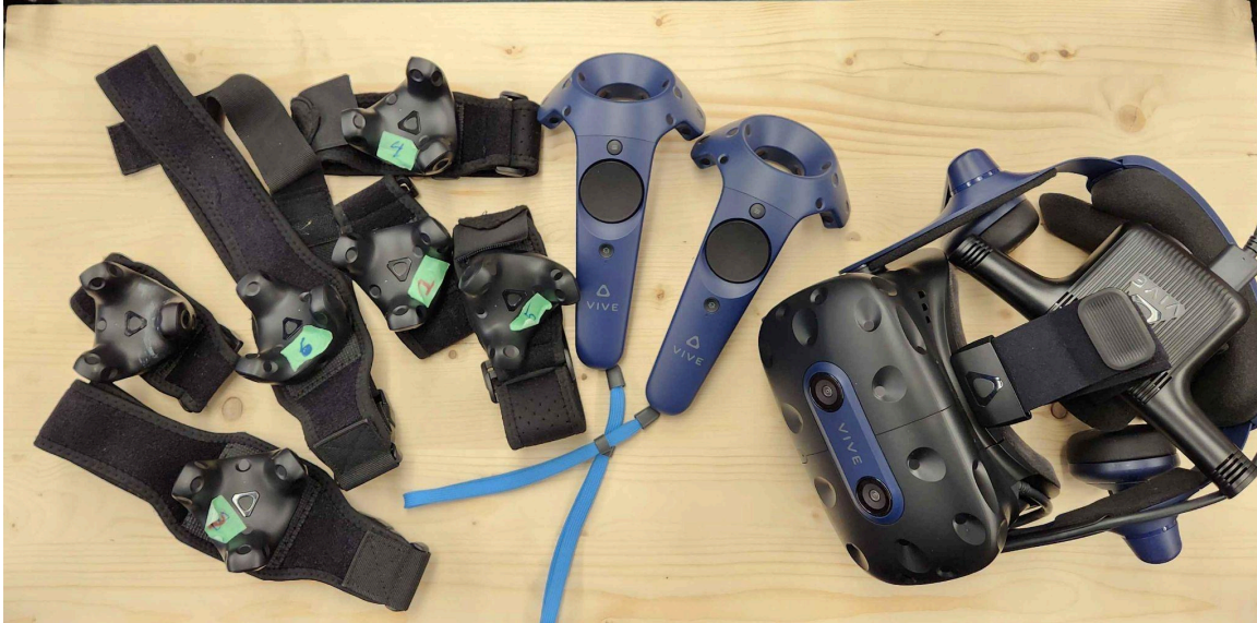
Figure 2.4. An image of an immersive VR bundle comprising the HTC Vive Trackers 3.0, Vive controllers, and the Vive Pro 2 HMD from left to right.
