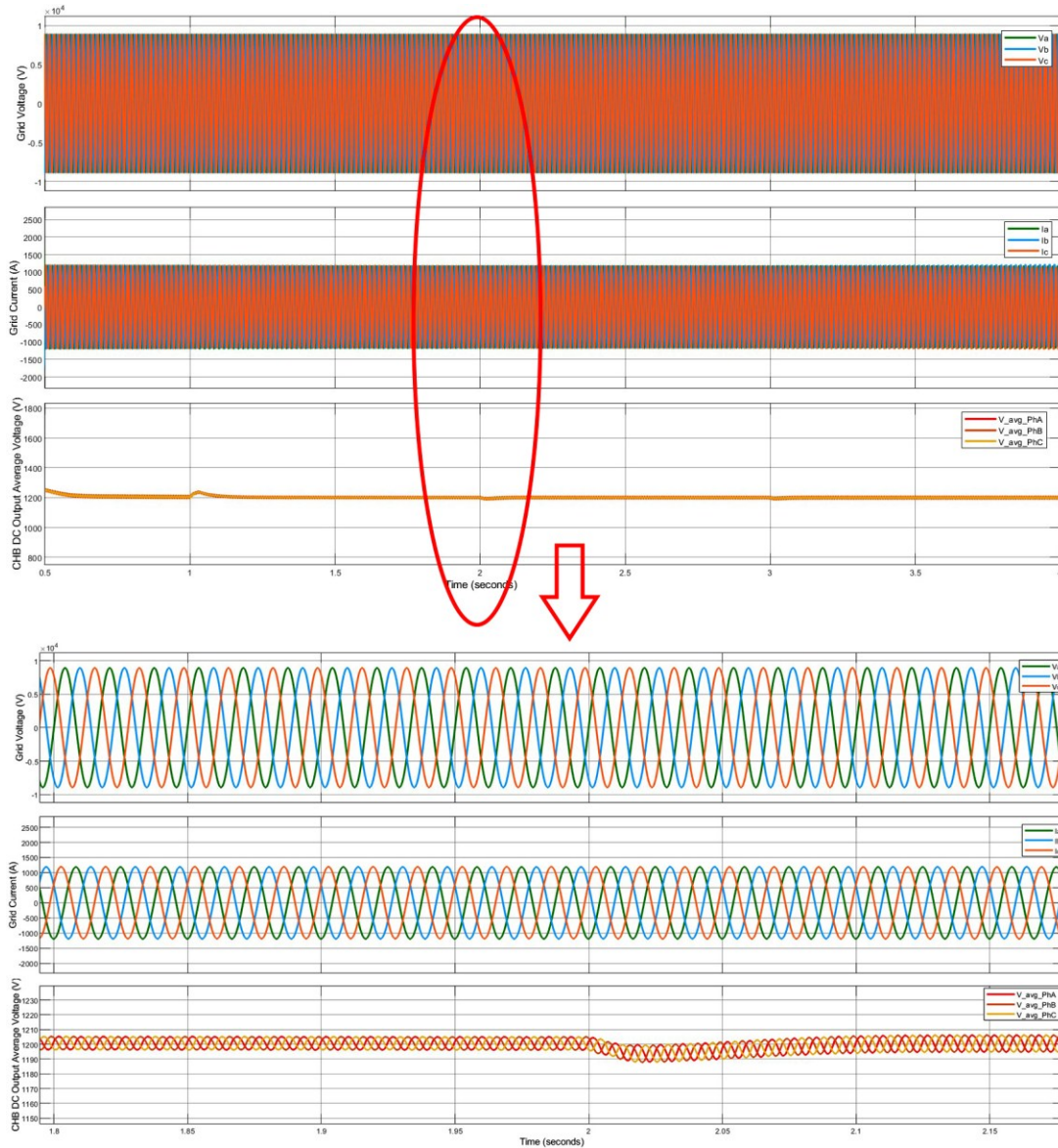
Figure 31: Grid voltage, grid current and average output DC voltage of CHB at each phase
